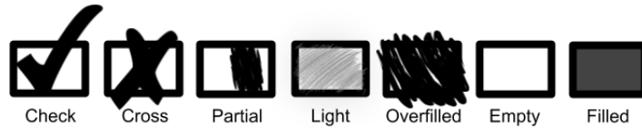
Fig. 3. Taxonomy of voter marks adapted from Bajcsy [2], including the five leftmost marks that may be considered marginal marks.
